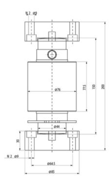
Technical drawing in mm with assembly kit.
